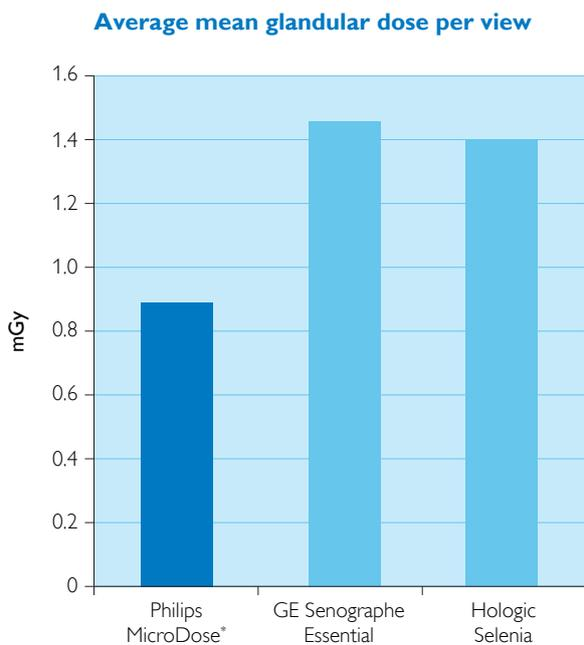
**Figure 3: Comparison of overall MGD for Philips MicroDose, GE Senographe Essential, and Hologic Selenia, based on BreastCheck 2009 data.**
